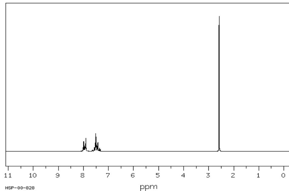
Molecular Formula  $\text{C}_8\text{H}_8\text{O}$ ,  $\delta$  7.9 = 2H,  $\delta$  7.3-7.7 = 3H,  $\delta$  2.6 = 3H.
