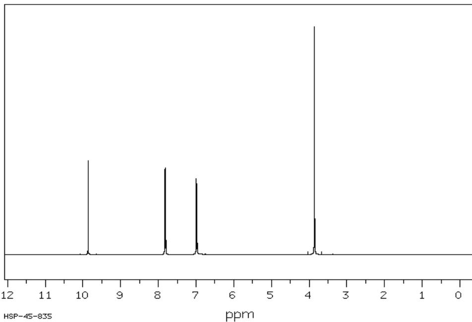
Molecular Formula  $\text{C}_8\text{H}_8\text{O}_2$ ,  $\delta$  9.9 = 1H,  $\delta$  7.8 = 2H,  $\delta$  7.0 = 2H,  $\delta$  3.9 = 3H.Spectrum (B):  $^1\text{H-NMR}$ , 90 MHz in  $\text{CDCl}_3$
