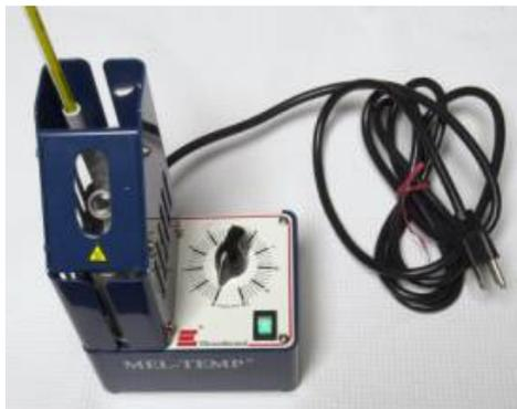
8. The identification of a unknown solid will be achieved by mixed melting point determination.
