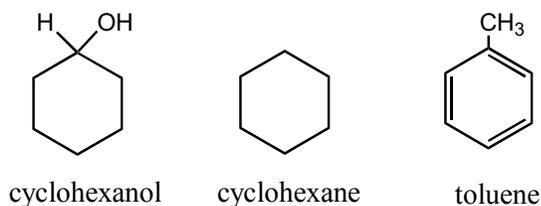
In Part B of this experiment, you will be given a 1:1 mixture of cyclohexane and toluene. You will fractionally distil the mixture, collecting first mainly the cyclohexane (fraction 1), then you will collect an intermediate second fraction containing the both cyclohexane and toluene, and finally a third fraction containing mainly toluene.
