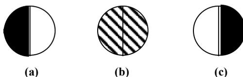
**Figure 7.4.** Possible views through the eyepiece of the polarimeter
