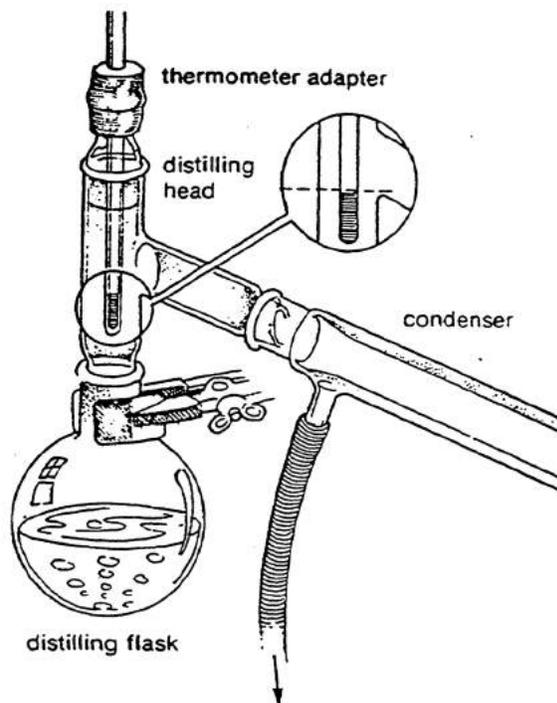
Figure 3.3. Thermometer placement during a simple distillation
