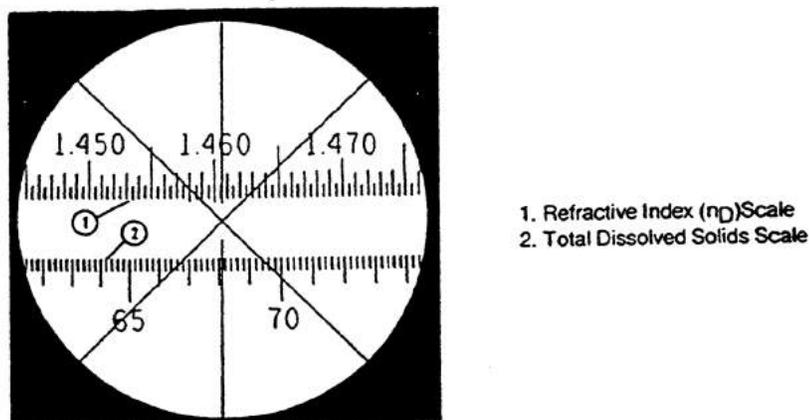
**Figure 4.5.** Reading the refractive index scale of an Abbé refractometer
