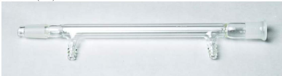
Distilling Column (Fractionation Column – without and with fractionating material, glass beads, inside)
