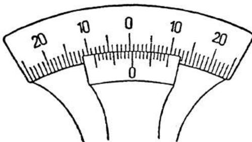
**Figure 7.5.** Reading the Vernier scale on the polarimeter
