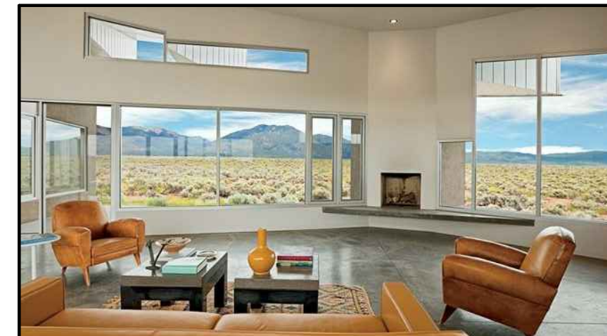
▲ Figure 35 (Antoine Predock Architect) Concrete floors at Sage House absorb heat let in by large windows.
