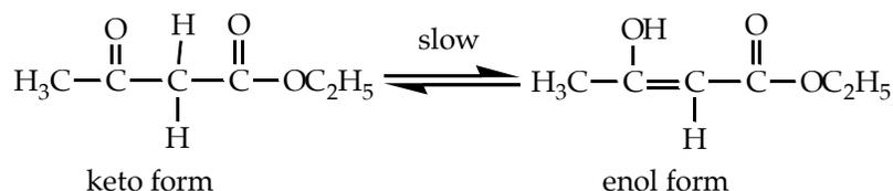
If a solution of iron (III) chloride is added to ethylaceto acetate, a coloured solution is obtained due to a reaction between the enol form and the iron (III) chloride.
