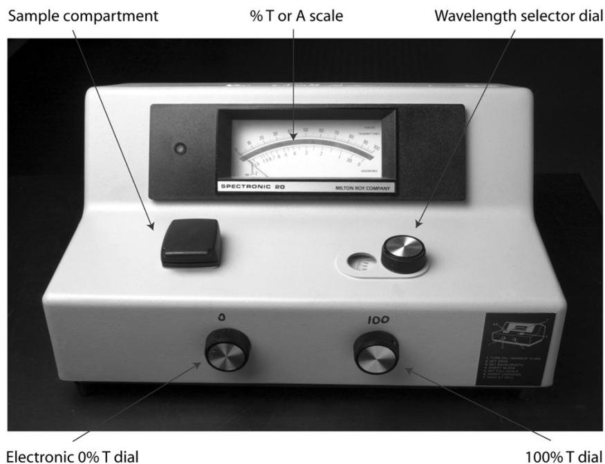
**Note:** When inserting the BLANK and UNKNOWN cuvettes into the spectrophotometer, be sure that the outside of the cuvette is clean and dry by polishing the glass with a tissue. Also place the cuvettes in the sample compartment in the same orientation each time.
