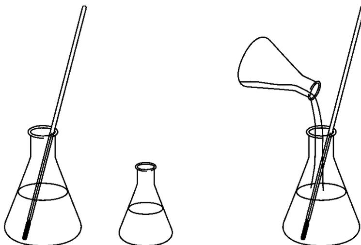
125 mL Erlenmeyer flask containing potassium iodide, sodium thiosulfate, starch indicator, and (if necessary) potassium chloride. The reaction vessel.
